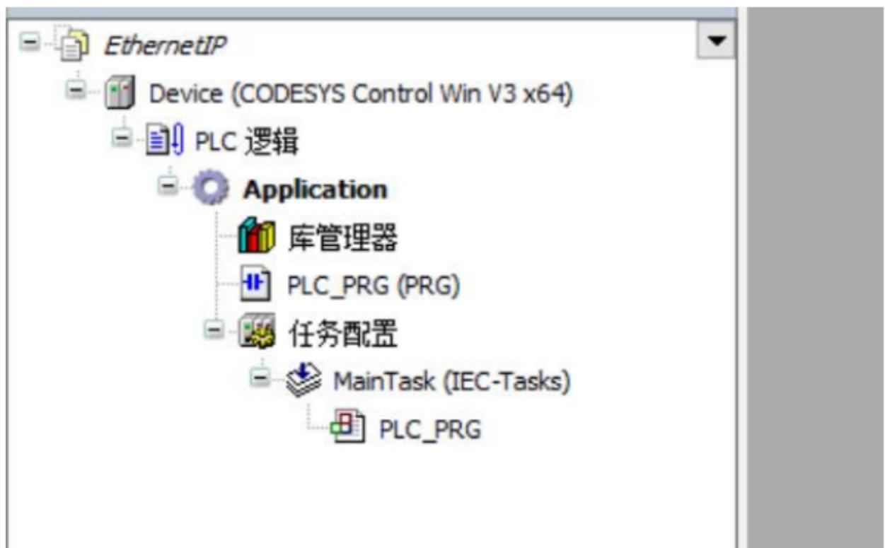
5. **Double-click "Device CODESYS Control Win V3 x64", click "Scan Network" on the right, select the correct network path, and click "Confirm".**
