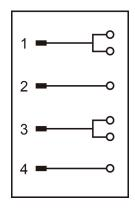
Pins 1 and 3 are power bits, which can be connected to the power cords of the two cables a and b respectively.
